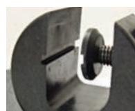
Clamp with grooves to hold calipers securely
