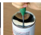
Piercing empty spray can for safe disposal
