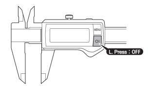
Power will automatically turn OFF after about 8 minutes with no activity. Press the Power Button or move the Slide to turn ON. The  $\square \square$  icon will display when the battery level is low. Please replace the battery.
