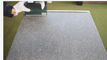
Measurement time is reduced to 1/8 compared with a conventional spirit level.
