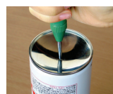
Piercing empty spray can for safe disposal
