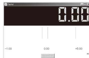
In Single Receive mode, the displayed measurement value changes only when the [SET] Button is pressed.
