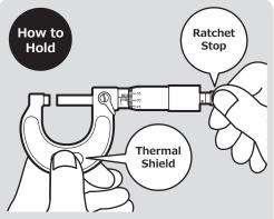
Grip the Micrometer on the Thermal Shield to prevent thermal expansion from body heat, and use the Ratchet Stop for consistent meas. force.
