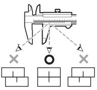
Read the Scale from directly above the Calipers. If the Scale is viewed at
