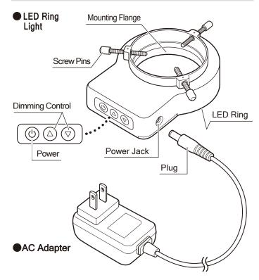
MOUNTING \*\*Follow the steps for proper installation on microscope.
