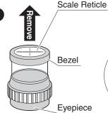
**%LSL-26** Reticle and Bezel are a single unit, please replace as pair without removing Reticle from Bezel
