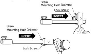
Loosen Arbor Lock Screw and insert Instrument Stem, and secure.
