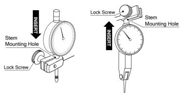
$\triangle$  NOTICE  $\bigcirc$  Be careful not to over tighten the Lock screw.
