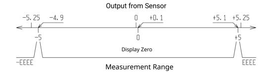
Reference point moved 2 mm/m using the 0-Cal, 1/2-Cal operations.
