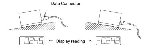
The display can be set to show the angle in units of DEG (°), or in units of mm/m (height difference in mm over 1 m.)
