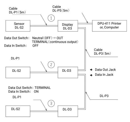
Data Out Switch: TERMINAL Data In Switch: OFF
