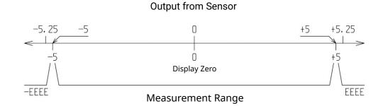
◎ Reference point moved 0.1 mm/m using the 0-Cal, 1/2-Cal operations. (For example, initial reading was 0.1 mm/m when 0-Cal is performed, or 0.20 mm/m before 1/2-Cal is performed.)
