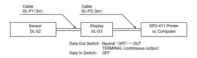
If the Data In Switch is in the ON position, "NO CONNECT" will be output to indicate that there was no data present on the Data In Jack.
