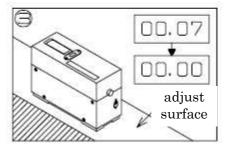
Leveling in two directions (X, Y direction)
