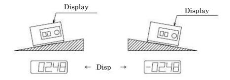
The Gauge will display the angle of inclination as mm/m, which is the elevation for the surface over a distance of 1 meter.
